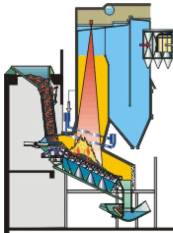
**Figure 2 – Martin reverse acting grate with combustion chamber and boiler**
